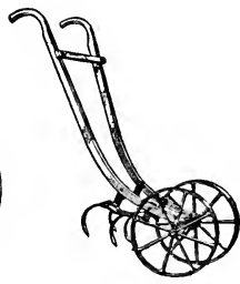
17. Double wheel-hoe, useful in straddling the row.
